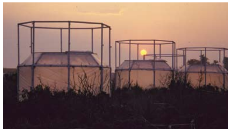
Plexiglass chambers at Kennedy Space Center allow researchers to gauge effects of climate change by exposing plots of scrub oaks to carbon-enriched air.
