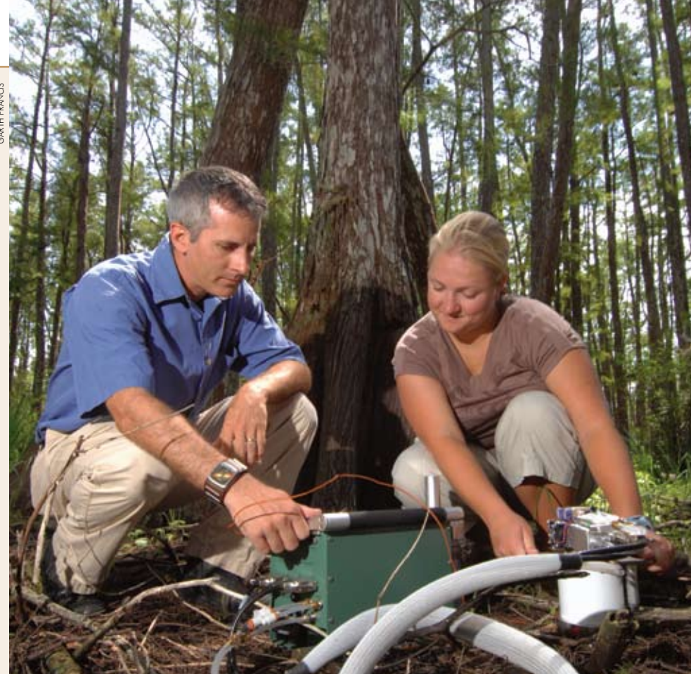
FGCU Assistant Professor Brian Bovard and junior Sarah Larsen use an infrared gas analyzer to monitor carbon dioxide and water vapor uptake and losses from soils, stems and leaves.
